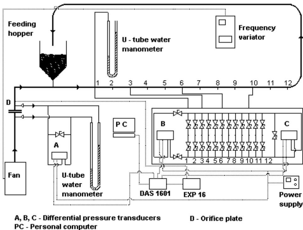
Figure 1 - Schematic diagram of the experimental apparatus.
