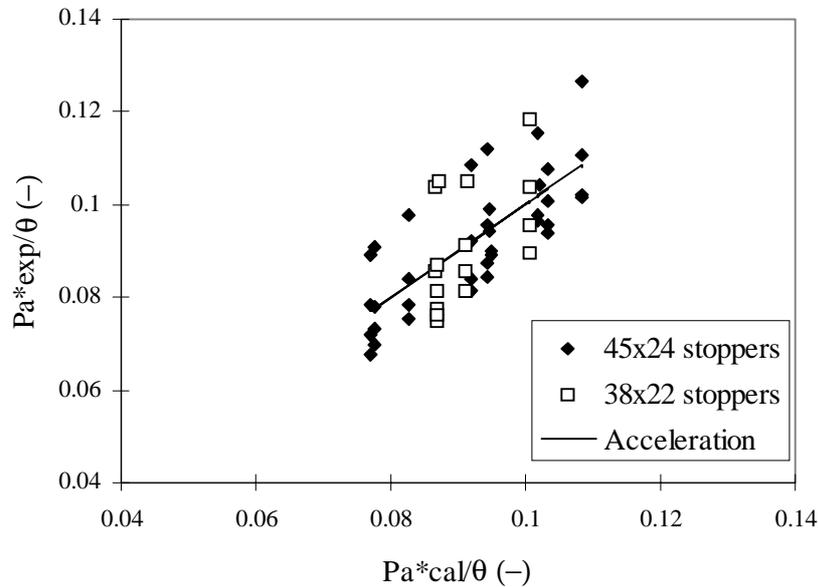
Figure 3 - Comparison between calculated specific acceleration pressure drop and experimental values obtained in parts of the acceleration region.
