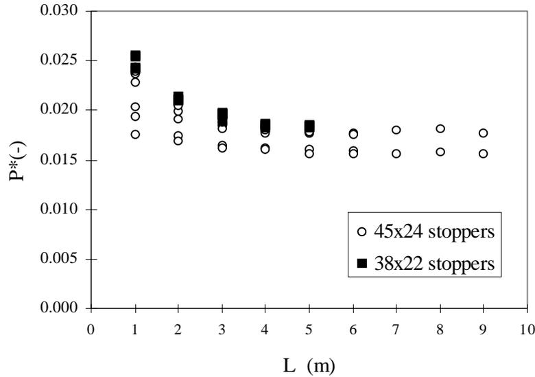
Figure 2 - Evolution of total pressure drop in the acceleration region.
